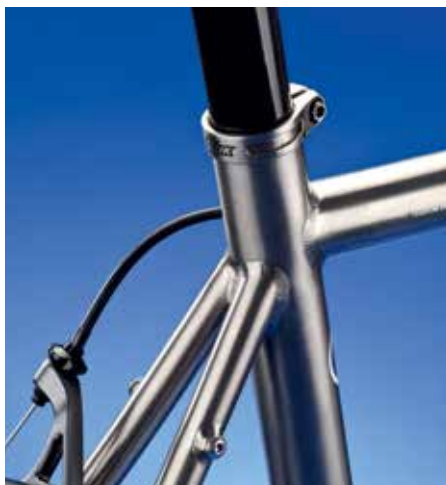
Weld quality was the best on test, while bowed seatstays (above) act as built-in shock absorbers. The stunning tapered head tube (right) looks like a metal hourglass
